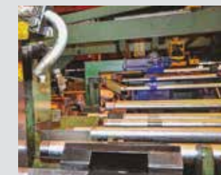
Extraction system of tubes from molten bath of zinc during hot dip galvanising of tubes
