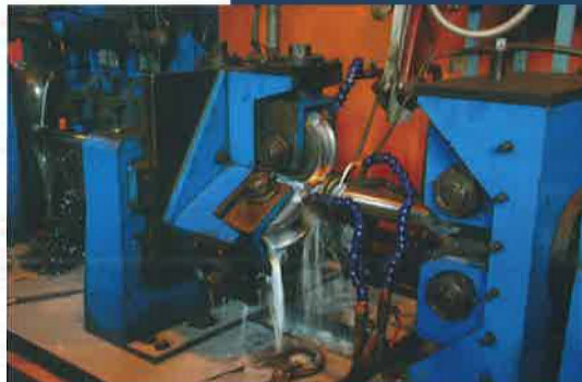
ELECTRIC WELDING OF SEAMS
